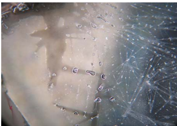
Figure 9: Optical micrograph at 50X magnification of LC solution heated at 70°C
