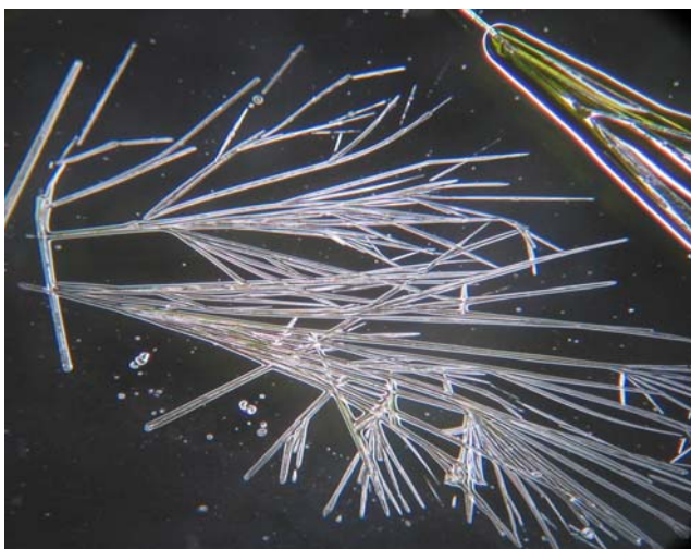
Figure 4: Optical micrograph at 50X magnification of as-prepared LC solution
